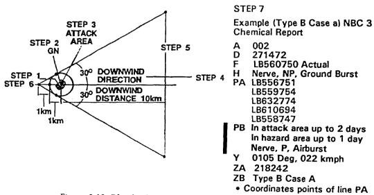
Figure 3-15. Plot for downwind hazard, Type B Case a.
